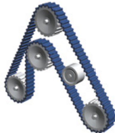
Figure 3.2.2: Multi-pulley drive with inside, smooth cylindrical pulley
