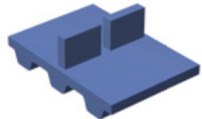
Figure 6.5.4: Rectangular cleats, arranged in series
