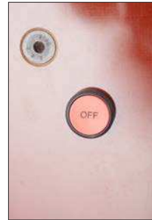
Fig.18 – Emergency STOP button at the front of the coil
