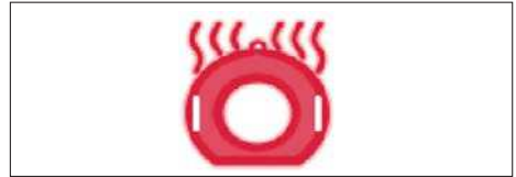
Fig.17 – Too hot coil warning symbol
