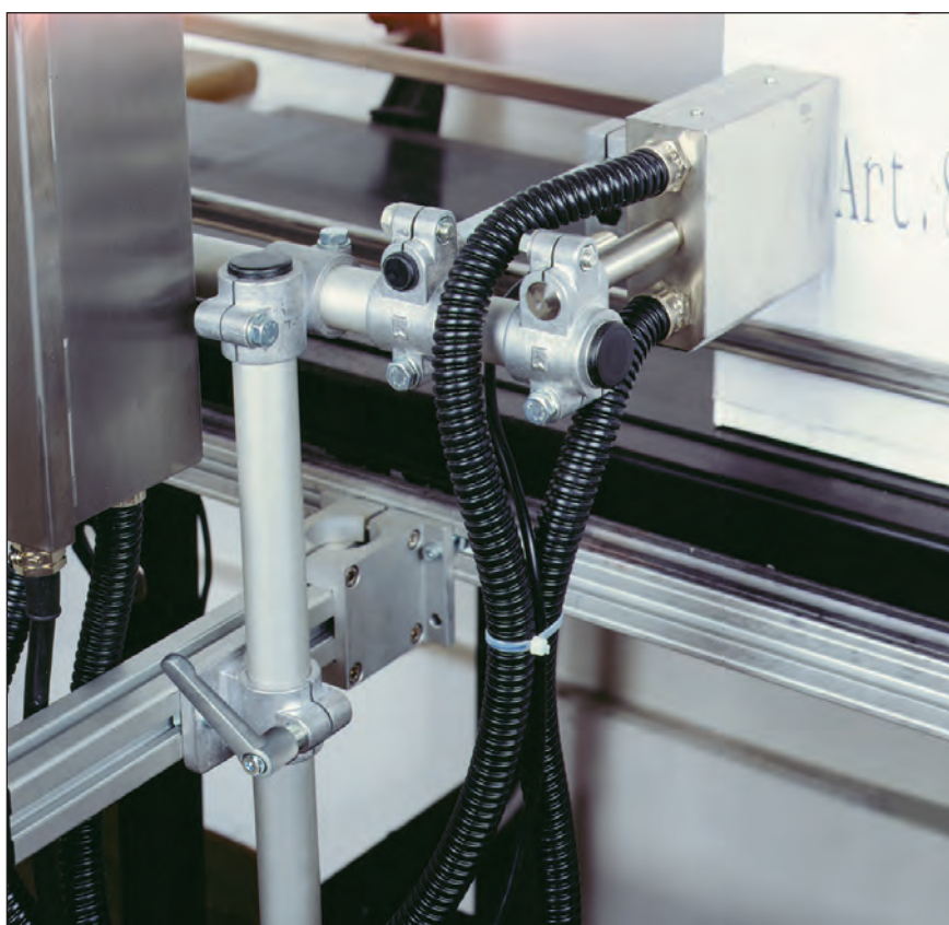
Print head holder on a packaging machine – can be moved as required.
