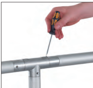
Release stopper with a screwdriver
